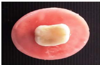
Figure 7 a: TOOTH EMBEDDED IN ACRYLIC RESIN BLOCK FOR FRACTURE RESISTANCE TESTING
