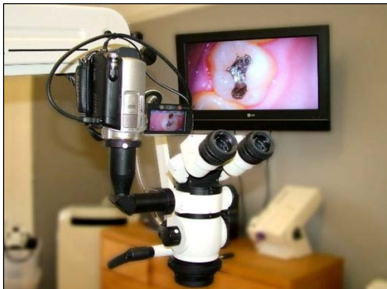
Figure 6: Microscope attached with SLR or video camera for communication
